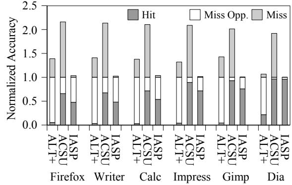
Figure 6: Prediction accuracy normalized to the total number of spin-ups with the buffer cache.
